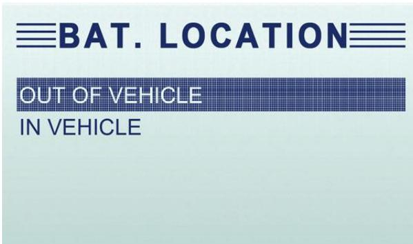
2. Scroll with the **UP** or **DOWN** button to highlight **OUT OF VEHICLE** or **IN VEHICLE** from BATTERY LOCATION menu and press **ENTER** to select the battery location.
