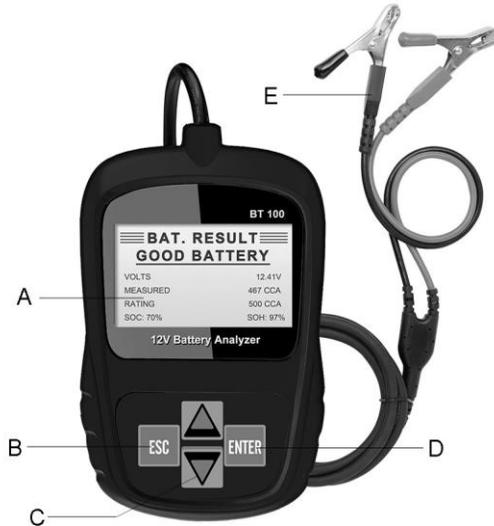
**A LCD Display** - shows menus, test results and operation tips.
